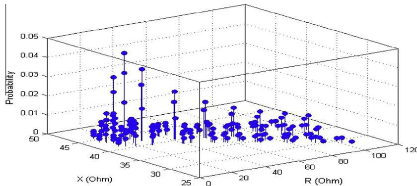
Fig. 5. Apparent impedances and their corresponding probabilities for a SG fault at 0.8 length of line 1-2.
