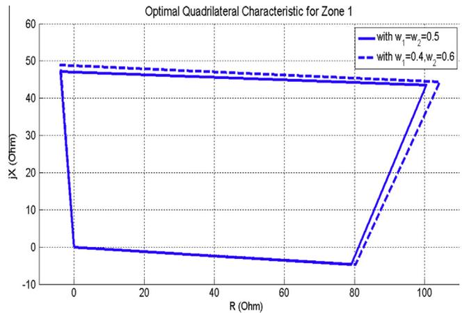
Fig. 8. Optimal setting of zone-1 for two cases of  $w_1$  and  $w_2$ .
