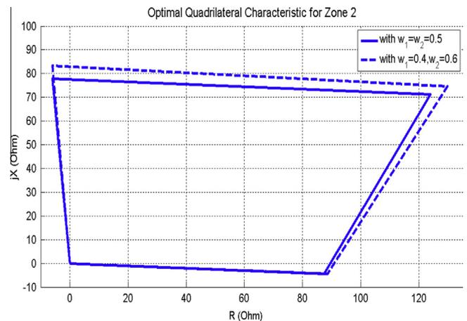
Fig. 9. Optimal setting of zone-2 for two cases of  $w_1$  and  $w_2$ .
