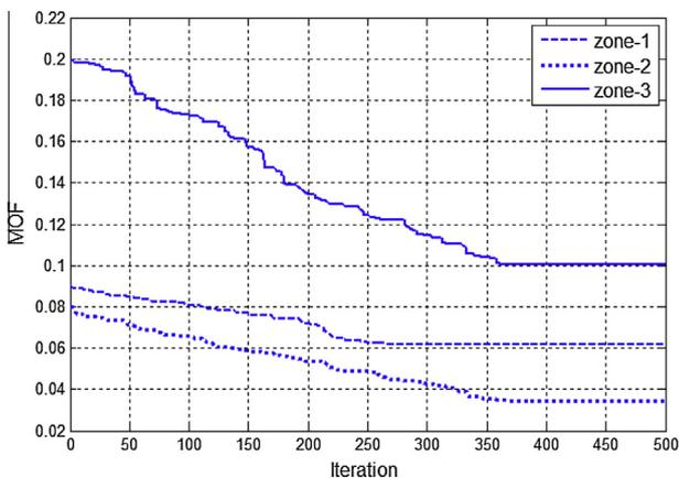
Fig. 7. The convergence plot of the GA for obtaining optimal characteristic of three zones.
