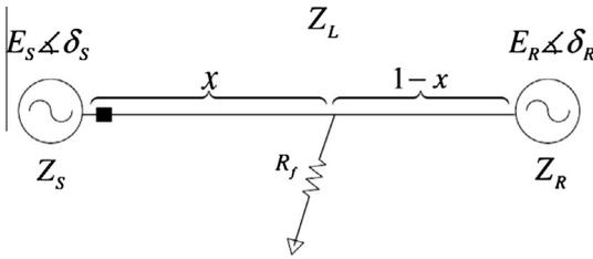
Fig. 1. Equivalent power system.
