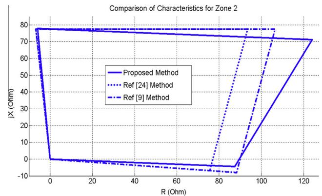
**Fig. 12.** Characteristic from proposed method and two other methods for zone-2.
