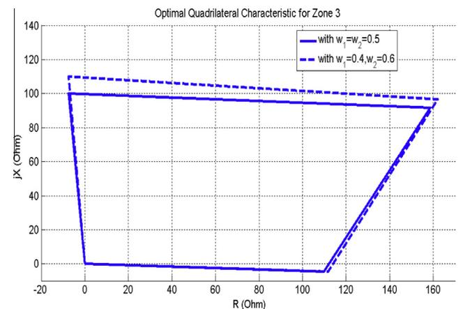
Fig. 10. Optimal setting of zone-3 for two cases of  $w_1$  and  $w_2$ .
