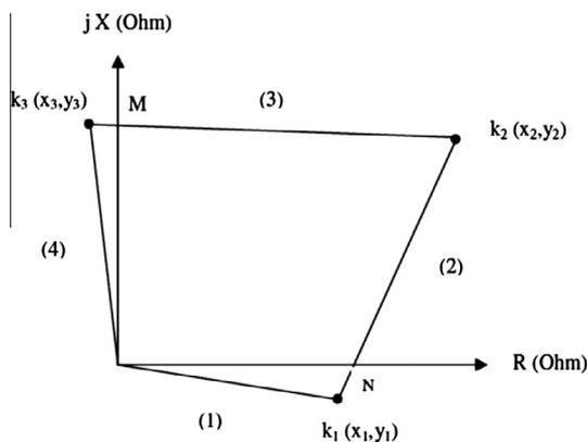
Fig. 2. Quadrilateral characteristic of distance relay.
