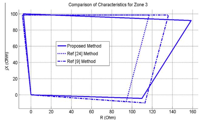
**Fig. 13.** Characteristic from proposed method and two other methods for zone-3.
