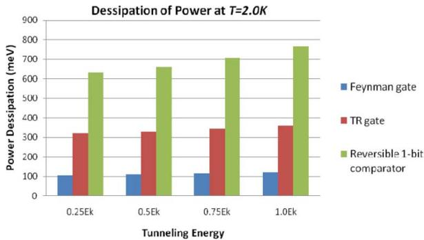
**Figure 11: Power dissipation of the proposed QCA layouts.**
