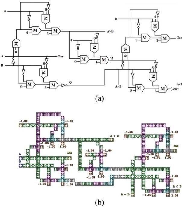
Figure 7: Proposed Feynman gate- and TR gate-based reversible 1-bit comparator (a) QCA schematic, (b) QCA layout.
