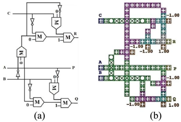
Figure 5: TR gate (a) QCA schematic, (b) QCA layout.
