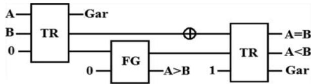
Figure 6: TR gate- and Feynman gate-based proposed reversible 1-bit comparator.
