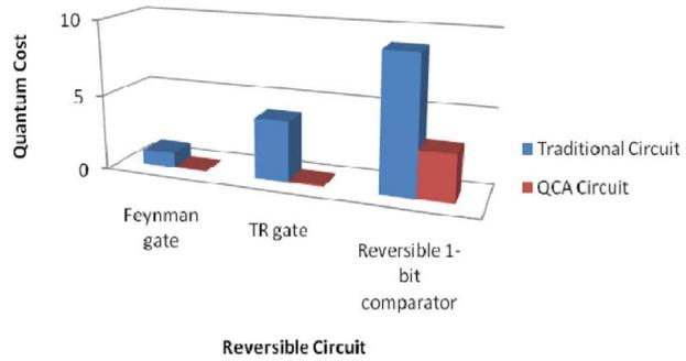
**Figure 10.** Quantum cost of the proposed conventional reversible comparator and QCA reversible comparator.
