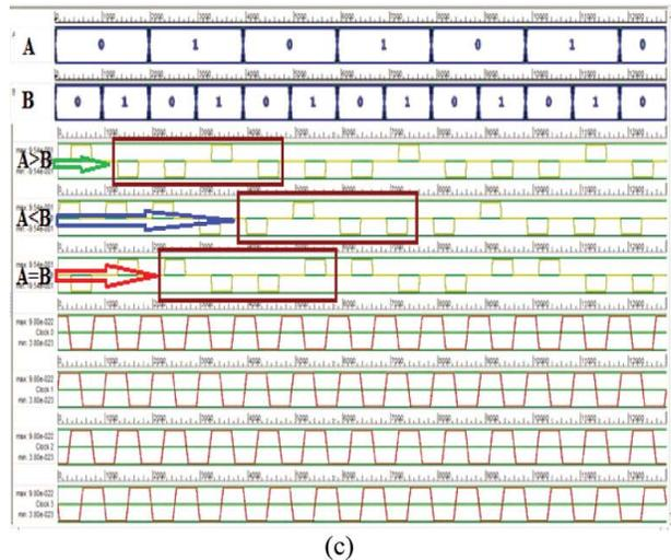
Figure 9: Simulation result of the proposed QCA circuit (a) Feynman gate, (b) TR gate, (c) 1-bit comparator.
