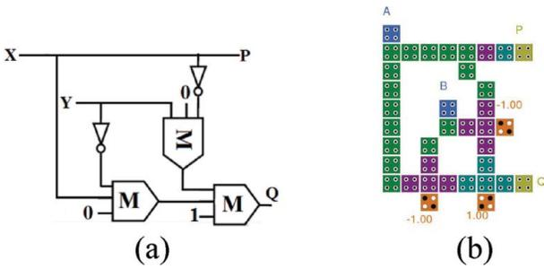
Figure 3: Feynman gate (a) QCA schematic, (b) QCA layout.
