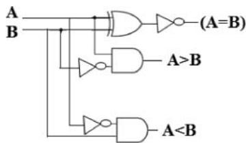
Figure 1: Logic circuit of 1-bit comparator.
