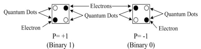
Fig. 1. QCA cell structure that generates logic 0 and logic 1.
