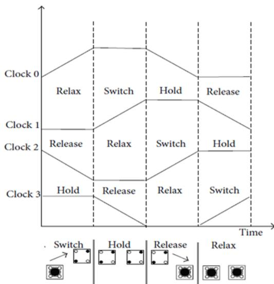
Fig. 3. The clock used in QCA.
