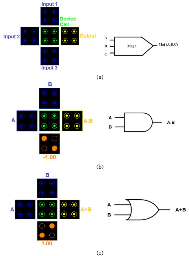
Fig. 5 (a) Three-input QCA majority function at left and the logical symbol at right. (b) and (c) AND and OR gates based on three-input QCA majority function.
