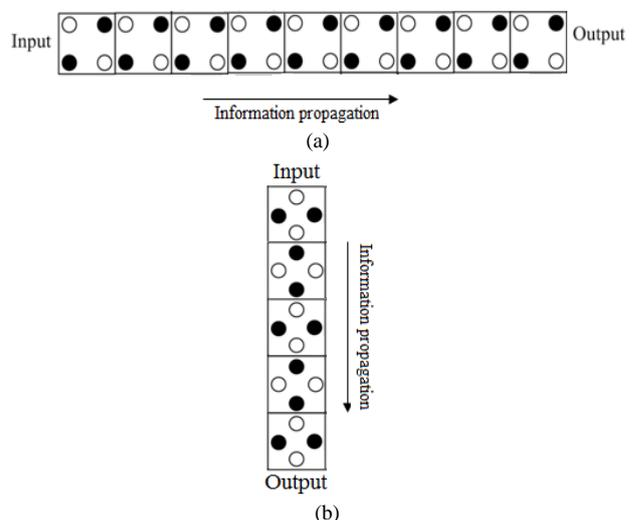
Fig. 2. Two types of QCA wire. (a)  $90^\circ$  QCA wire and (b)  $45^\circ$  QCA wire.
