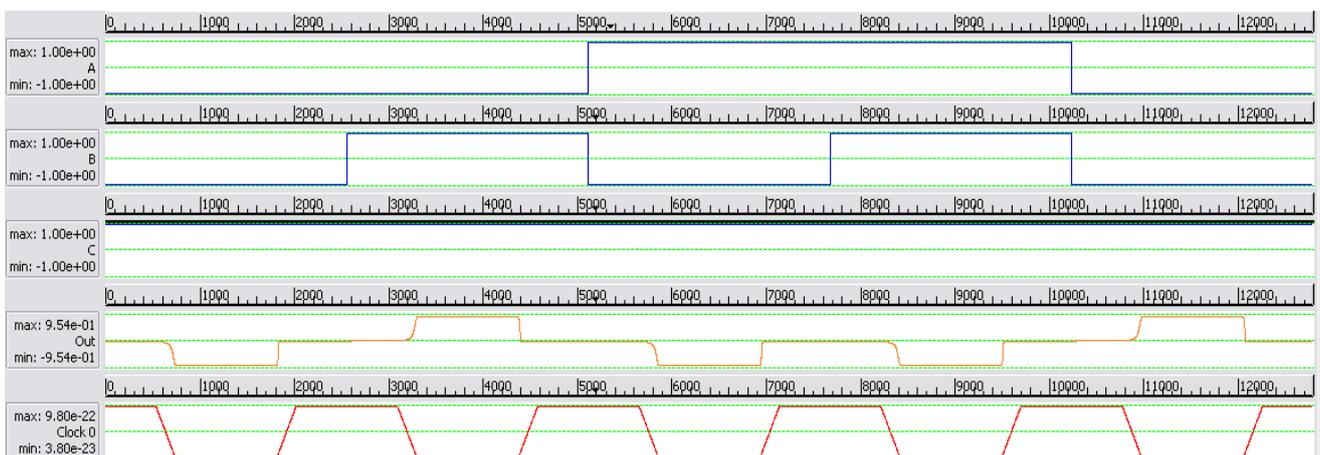
Fig. 8. The proposed full comparator simulation result. The first three waveforms are the inputs and the fourth one is the output. The last waveform is clock 0 which generates the output.
