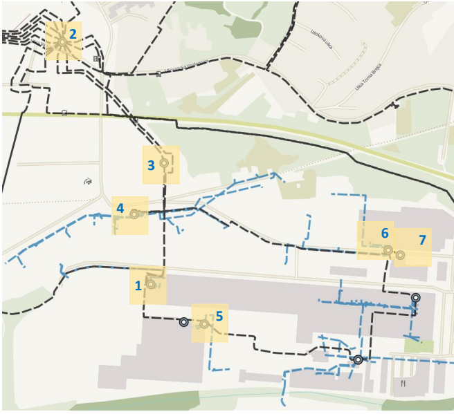
Fig. 2. SUNSEED Map: Electricity distribution network with PMU locations.
