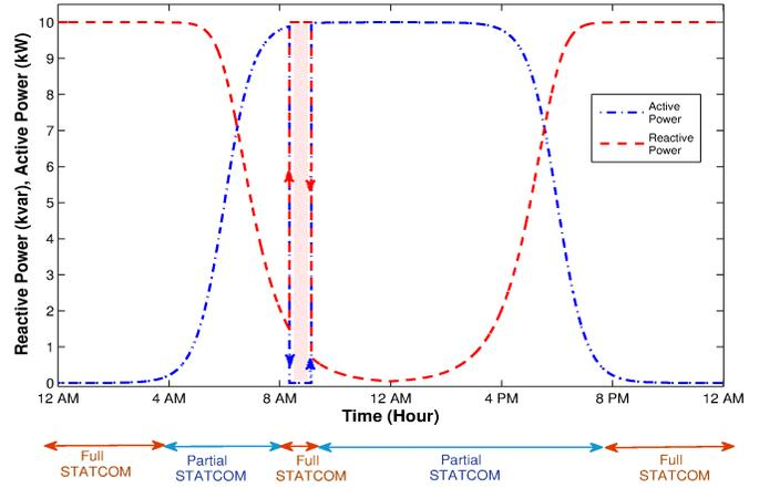
Fig. 1. Concept of smart PV inverter control as STATCOM
