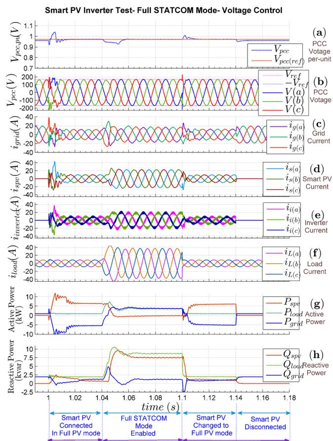
Fig. 4. Simulation results for full STATCOM mode with voltage control during daytime a) PCC voltage in per-unit b) PCC voltage c) Grid current d) Smart PV current e) Inverter current f) Load current g) Active power h) Reactive power
