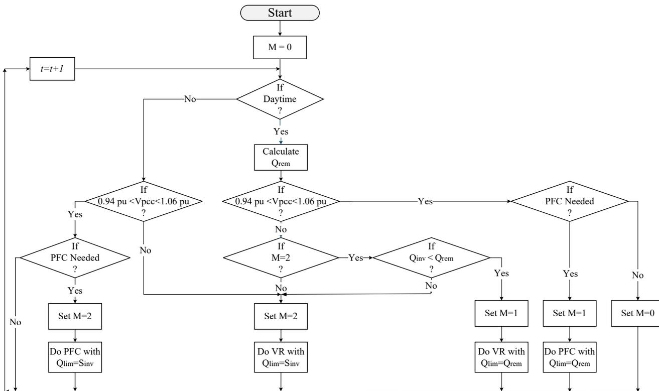
Fig. 3. Flowchart of the smart PV inverter operating modes
