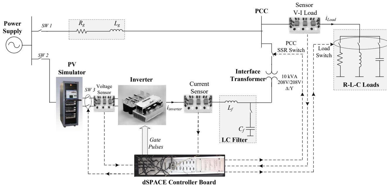
Fig. 8. Lab setup of the study system with the smart inverter PV-STATCOM
