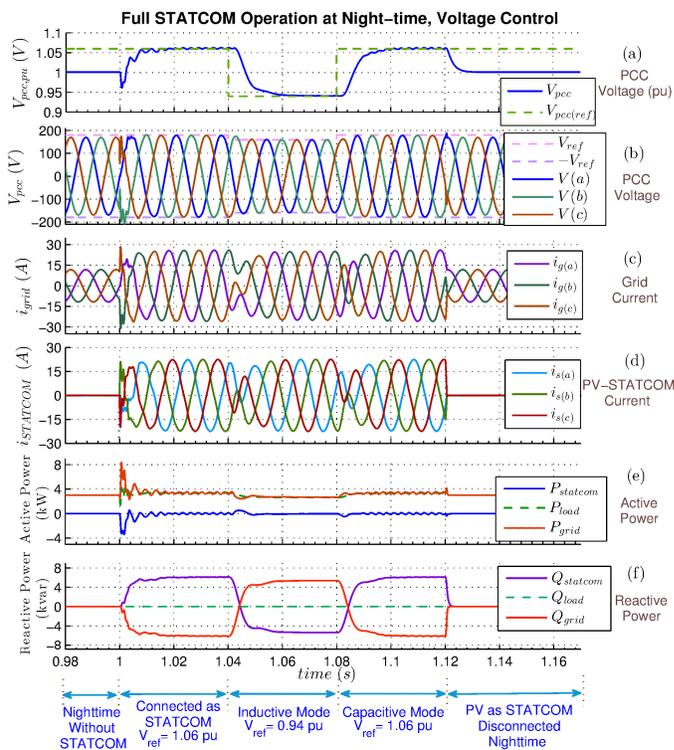
Fig. 5. Simulation results for full STATCOM operation with voltage control during nighttime a) PCC voltage in per-unit b) PCC voltage c) Grid current d) PV current e) Active power f) Reactive power
