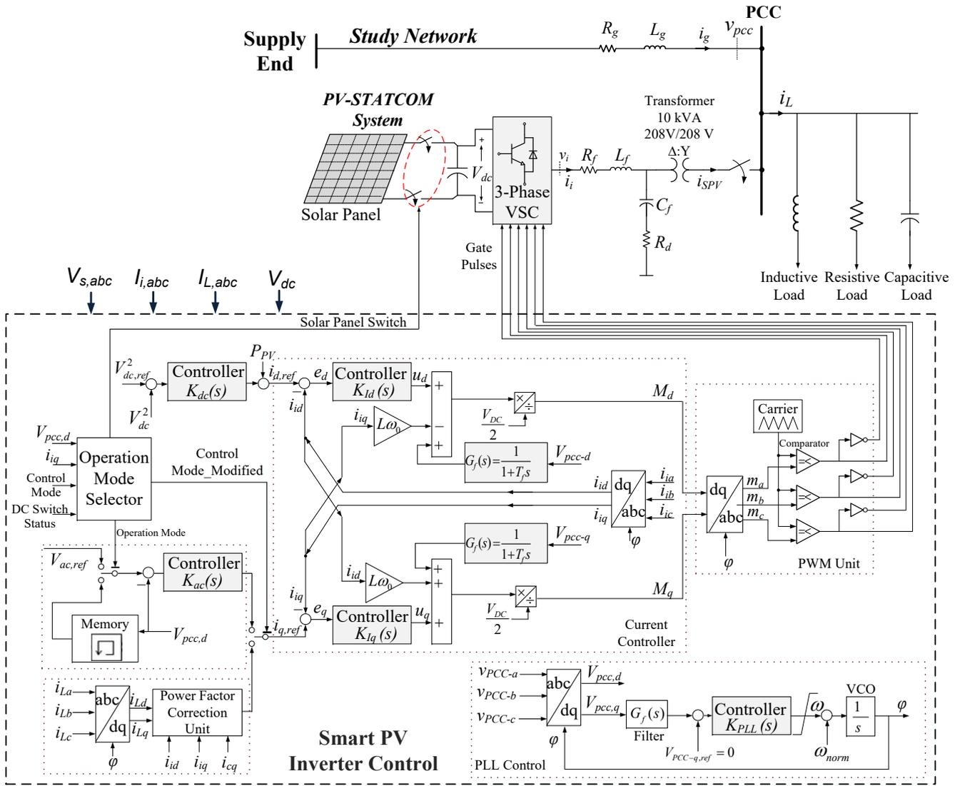
Fig. 2. Modeling of the study system and control components
