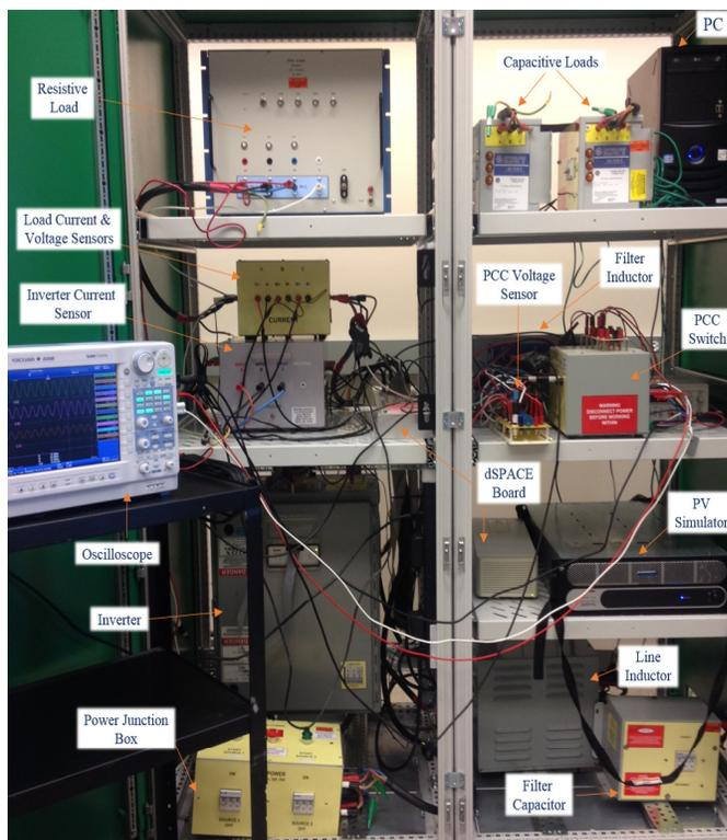
Fig. 9. Actual Lab setup of the study system with PV-STATCOM
