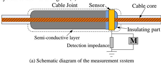
(a) Schematic diagram of the measurement system
