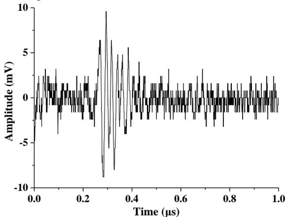
Figure 13 Waveform of the sensor at apparent discharge quantities of 10 pC
