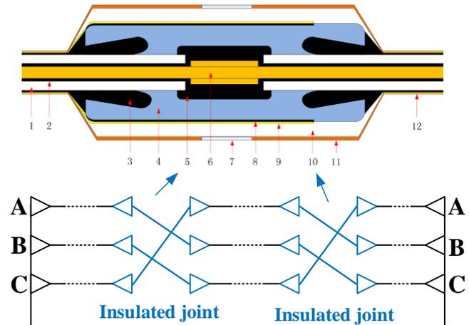
1- XLPE insulation; 2- inner semi-conductive layer; 3- stress cone; 4- silicone rubber insulation; 5- inner field control layer; 6- conductor and connector; 7- epoxy resin; 8- outer semi-conductive layer; 9- copper wire sleeve; 10- polyurethane sealant layer; 11- copper protection tube; 12- jacket.
