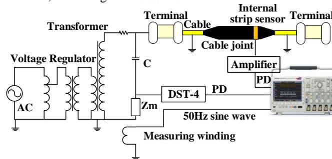
Figure 12 Partial discharge detection on the platform of 110 kV XLPE cable joints
