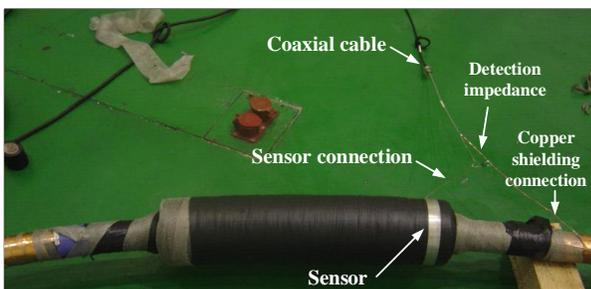
(b) Physical view of the measurement system
