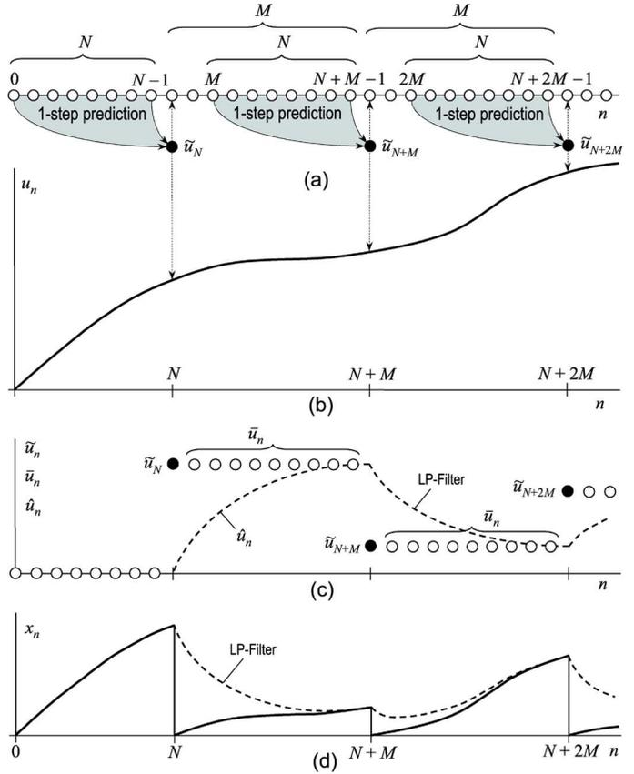
Fig. 5. GPS synchronization algorithm for  $M > N$ . (a) Time diagram. (b) Time error  $u_n$  of an unlocked clock. (c) Optimal predictive estimate  $\tilde{u}_n$ , hold filter output  $\bar{u}_n$ , and smoothed estimate  $\hat{u}_n$ . (d) Time error  $x_n$  of a locked clock. (Bold) piecewise and (dashed) smoothed by an LP filter.
