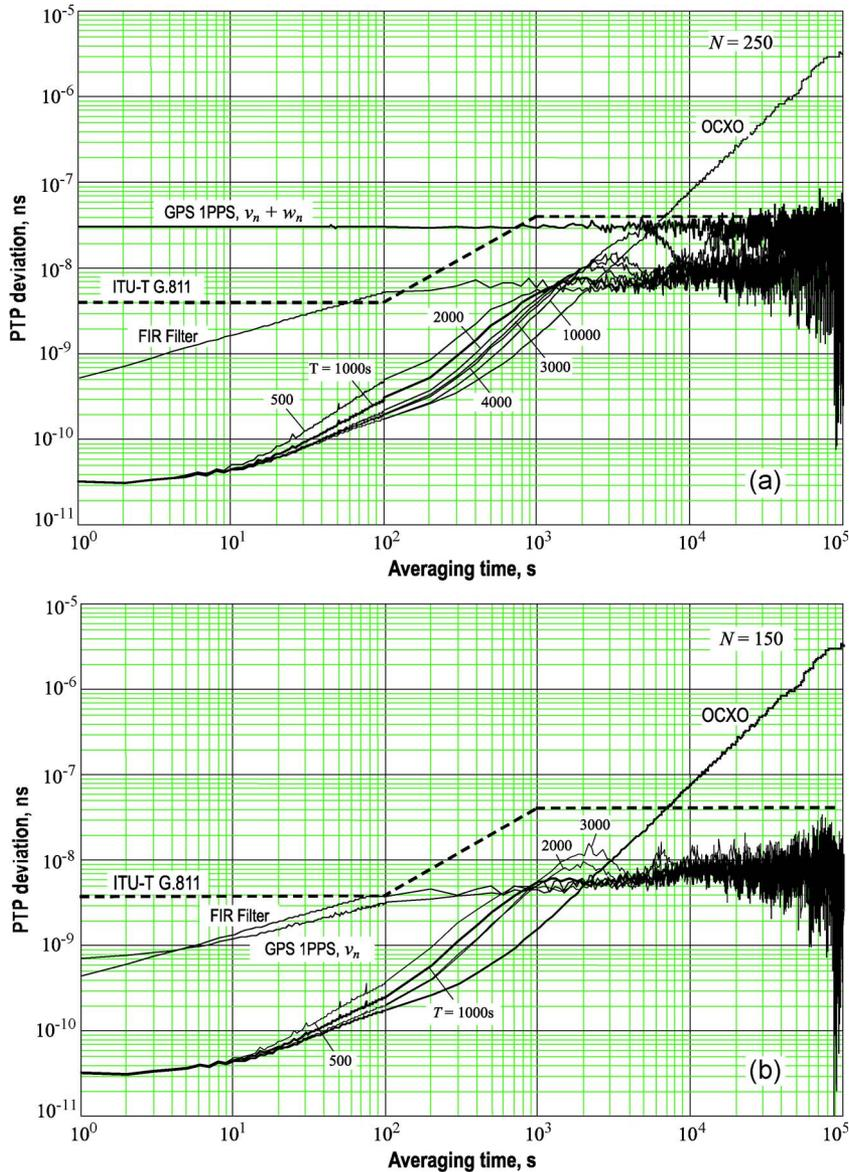
Fig. 10. PTP deviation of the GPS locked crystal clock for different  $T$ 's of the one-order LP filter. (a) Sawtooth measurement  $s_n = v_n + w_n$  with  $N_{opt} = 250$ . (b) Sawtoothless measurement  $s_n = v_n$  with  $N_{opt} = 150$ .
