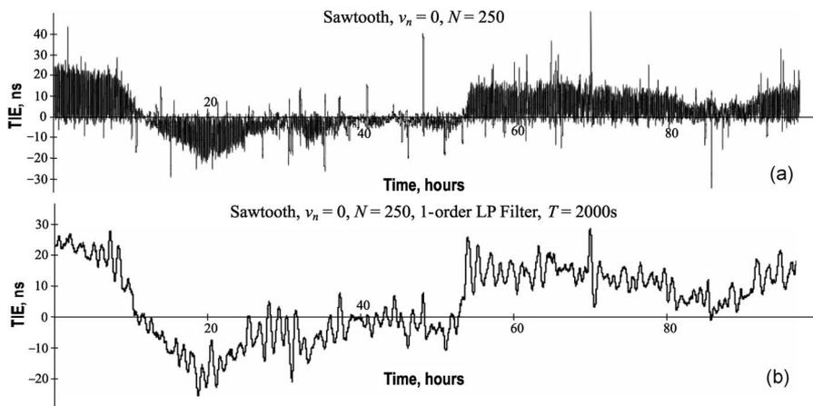
Fig. 8. Limiting time error  $x_n$  of the optimally GPS locked crystal clock with measurements without uncertainty, i.e.,  $s_n = w_n$ . (a) Piecewise steering with  $N = 250$ . (b) Smoothed steering with the one-order LP filter, i.e.,  $T = 2000$  s.
