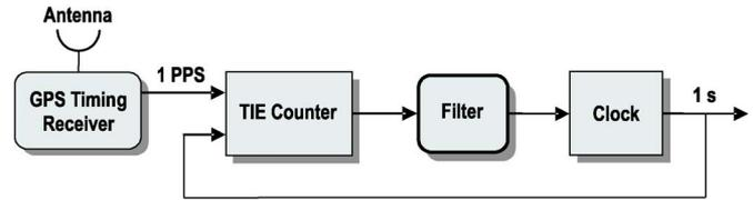
Fig. 1. Generalized structure of GPS disciplining of local clocks by the 1PPS timing signals.
