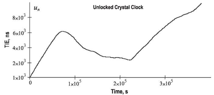
Fig. 4. Typical behavior of the TIE of an unlocked crystal clock.
