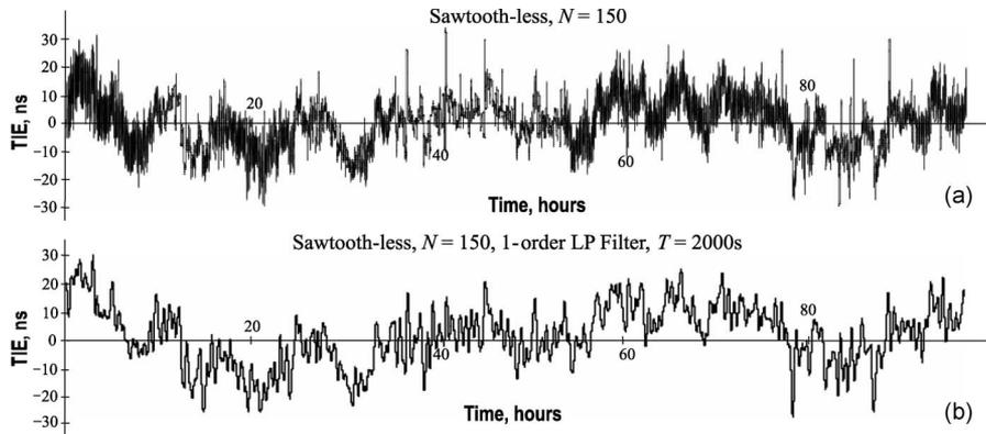
Fig. 7. Time error  $x_n$  of the optimally GPS locked crystal clock with sawtoothless measurements, i.e.,  $s_n = v_n$ . (a) Piecewise steering with  $N = 150$ . (b) Smoothed steering with the one-order LP filter, i.e.,  $T = 2000$  s.
