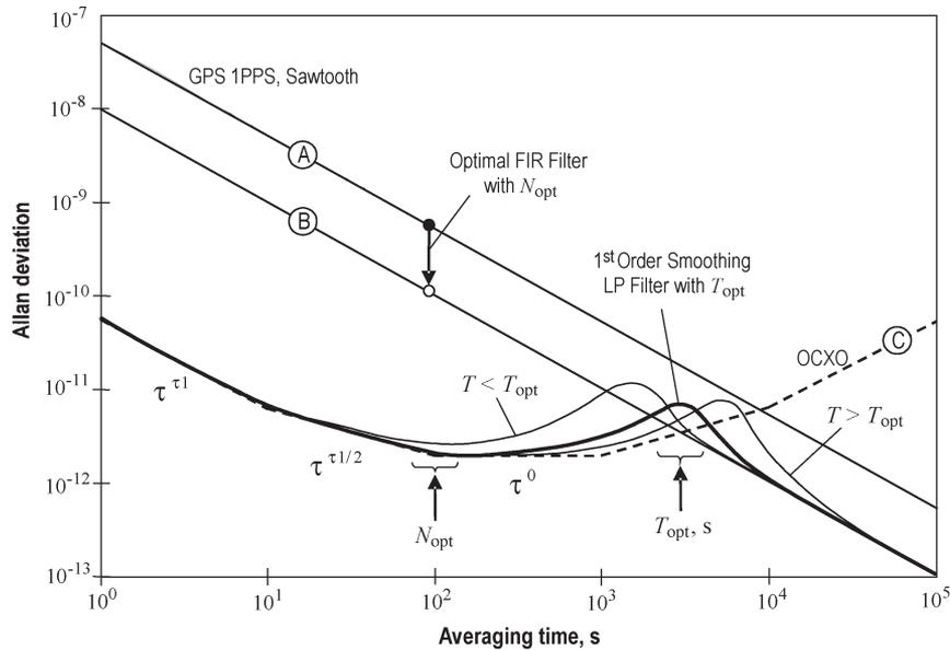
Fig. 11. Allan deviation of a local crystal clock synchronized by GPS 1PPS timing signals.
