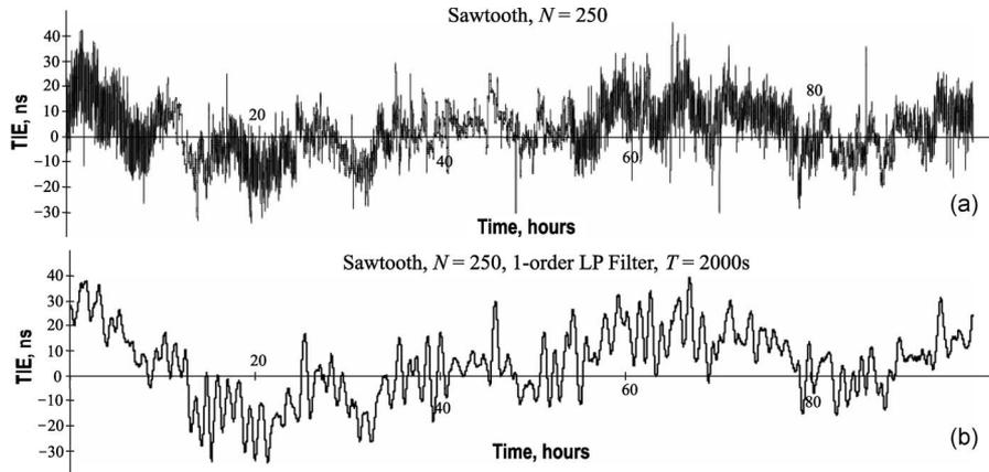
Fig. 6. Time error  $x_n$  of the optimally GPS locked crystal clock with sawtooth measurements, i.e.,  $s_n = v_n + w_n$ . (a) Piecewise steering with  $N = 250$ . (b) Smoothed steering with the one-order LP filter, i.e.,  $T = 2000$  s.
