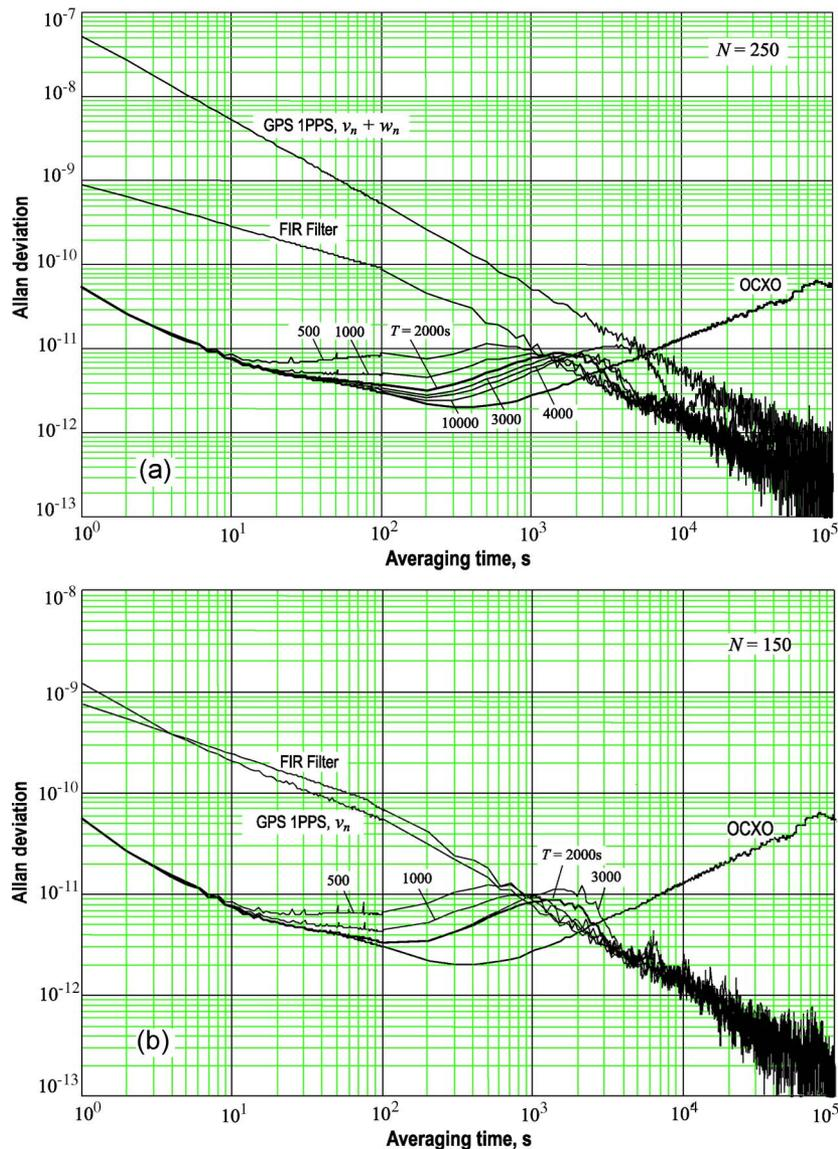
Fig. 9. Allan deviation of the GPS locked crystal clock for different  $T$ 's of the one-order LP filter. (a) Sawtooth measurement  $s_n = v_n + w_n$  with  $N_{opt} = 250$ . (b) Sawtoothless measurement  $s_n = v_n$  with  $N_{opt} = 150$ .
