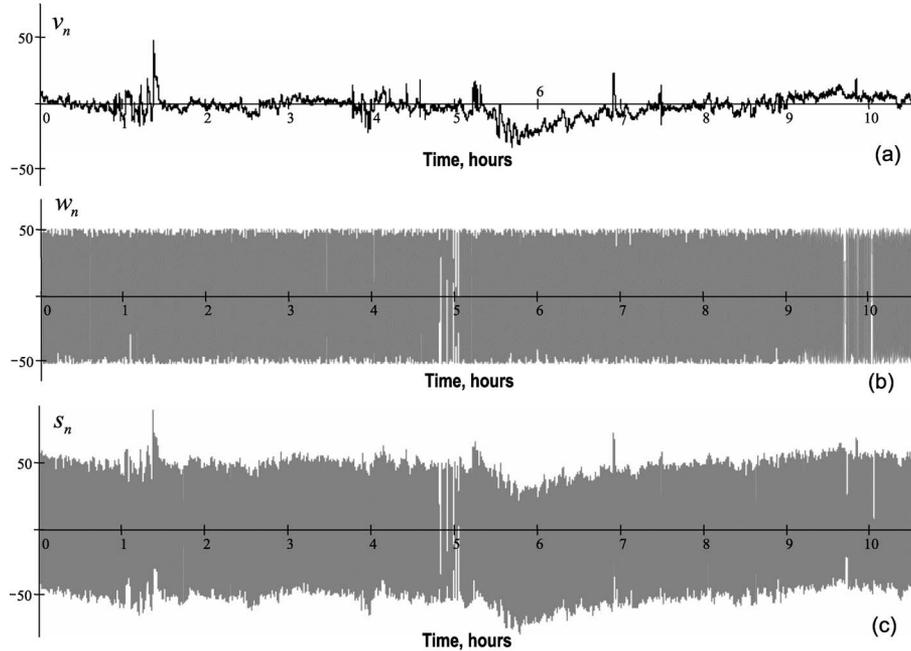
Fig. 3. Typical time errors of a Motorola-based GPS timing receiver. (a) Time uncertainty  $v_n$  caused by different satellites in a view and other random factors. (b) Sawtooth noise  $w_n$  induced by the receiver. (c) Time error  $s_n$  in the 1PPS reference signal.
