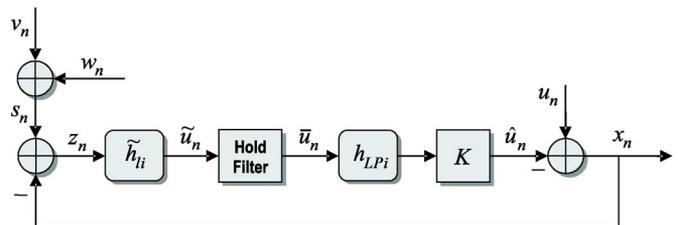
Fig. 2. Loop model of GPS synchronization of a local clock by the 1PPS timing signals.
