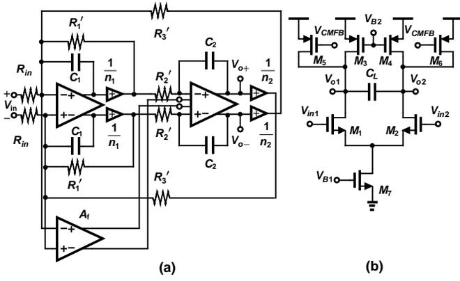
Fig. 3. (a) Biquad with the feedforward amplifier for noise cancellation (b) Feedforward amplifier (common mode feedback is not shown.)
