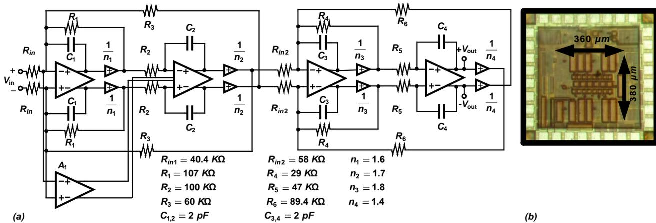
Fig. 7. (a) Fourth-order filter for Bluetooth application. (b) Microphotograph of the Bluetooth filter.
