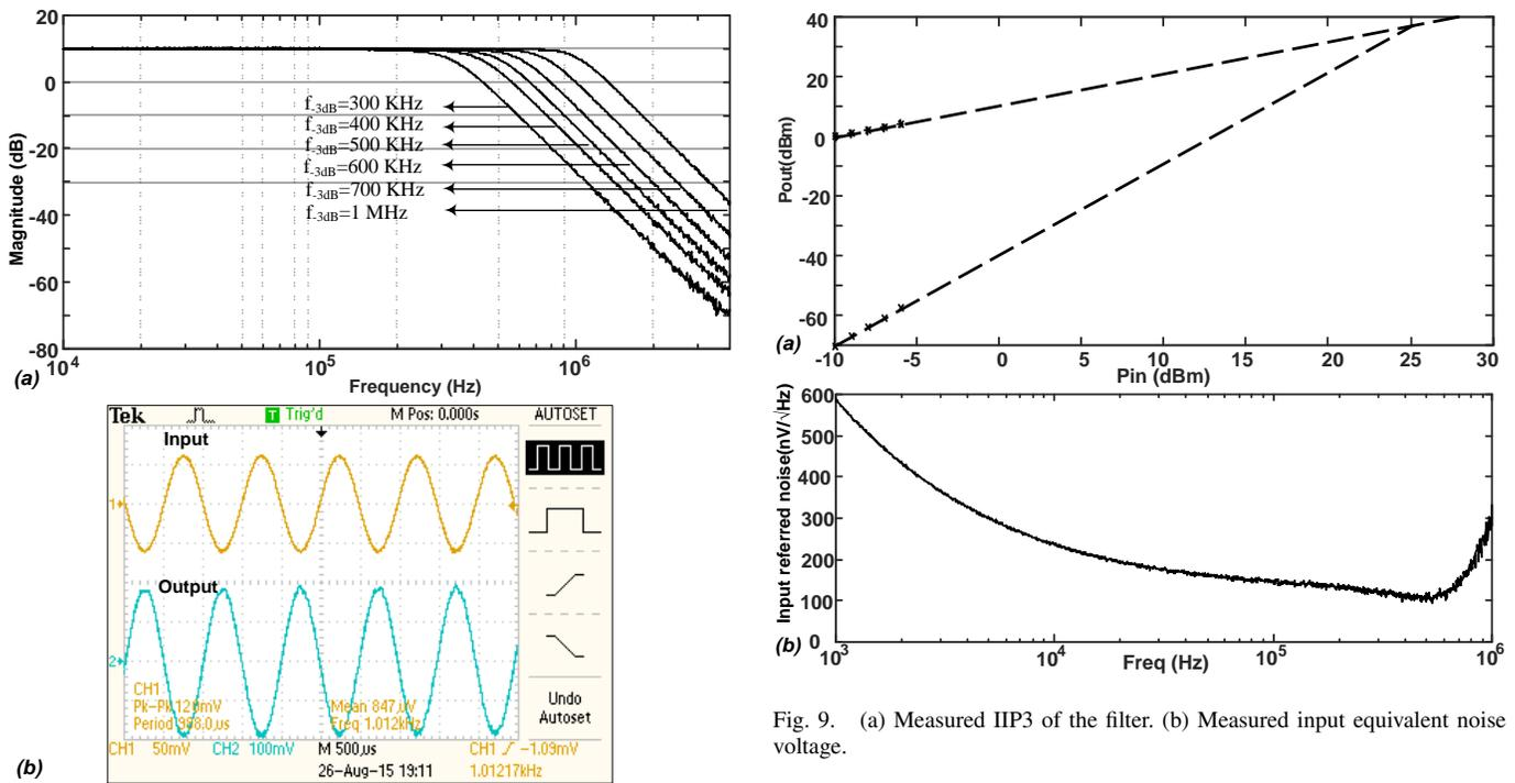
Fig. 8. (a) Frequency response of the filter. (b) Filter's output waveform for a 1 KHz, 60mV sinusoidal input voltage.
