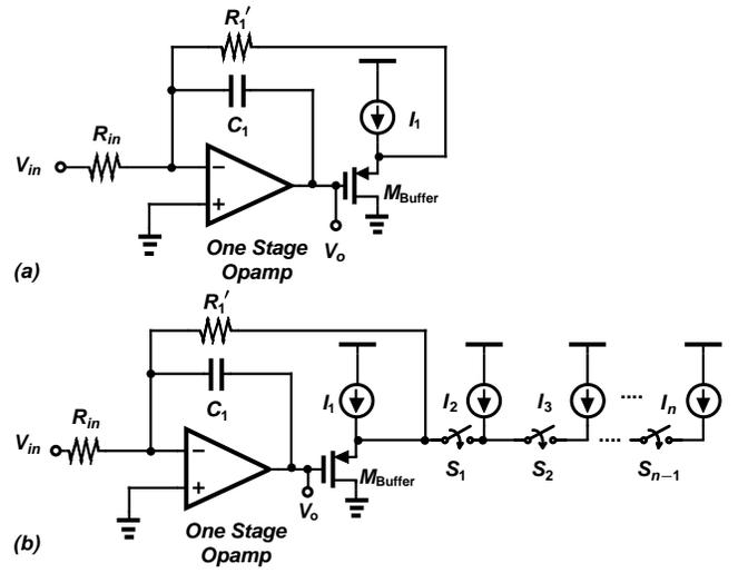
Fig. 5. (a) Source follower as  $\frac{1}{n}$  stage. (b) Tuning method for the integrator.
