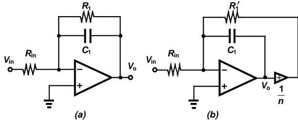
Fig. 1. (a) Lossy integrator (b) integrator with  $\frac{1}{n}$  at the output.
