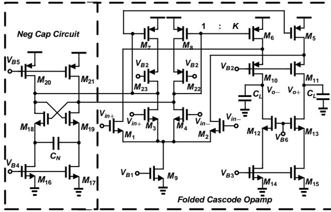
Fig. 6. Single-stage opamp with negative capacitance circuit for BW enhancement.
