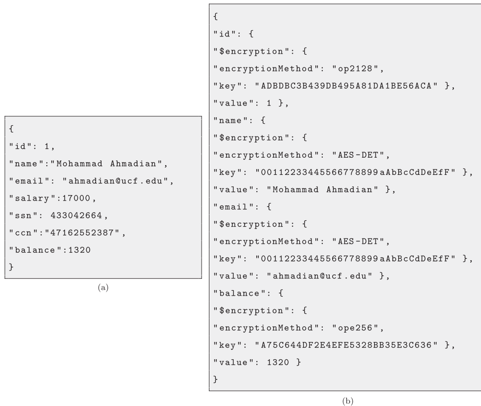
Fig. 9. The security plan for the sample input: (a) The data element section of sample security plan. (b) The output of the JSON data validation for the sample database.
