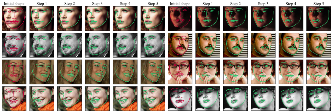
Fig. 4: Landmark localization for 5 recurrent steps. On the left, we show some examples, for which 5 recurrences are sufficient, while the examples on the right require additional recurrences.
