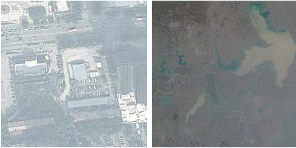
Fig. 1. Example of hazy satellite images. As can be seen that poor contrast makes target detection and image interpretation difficult.
