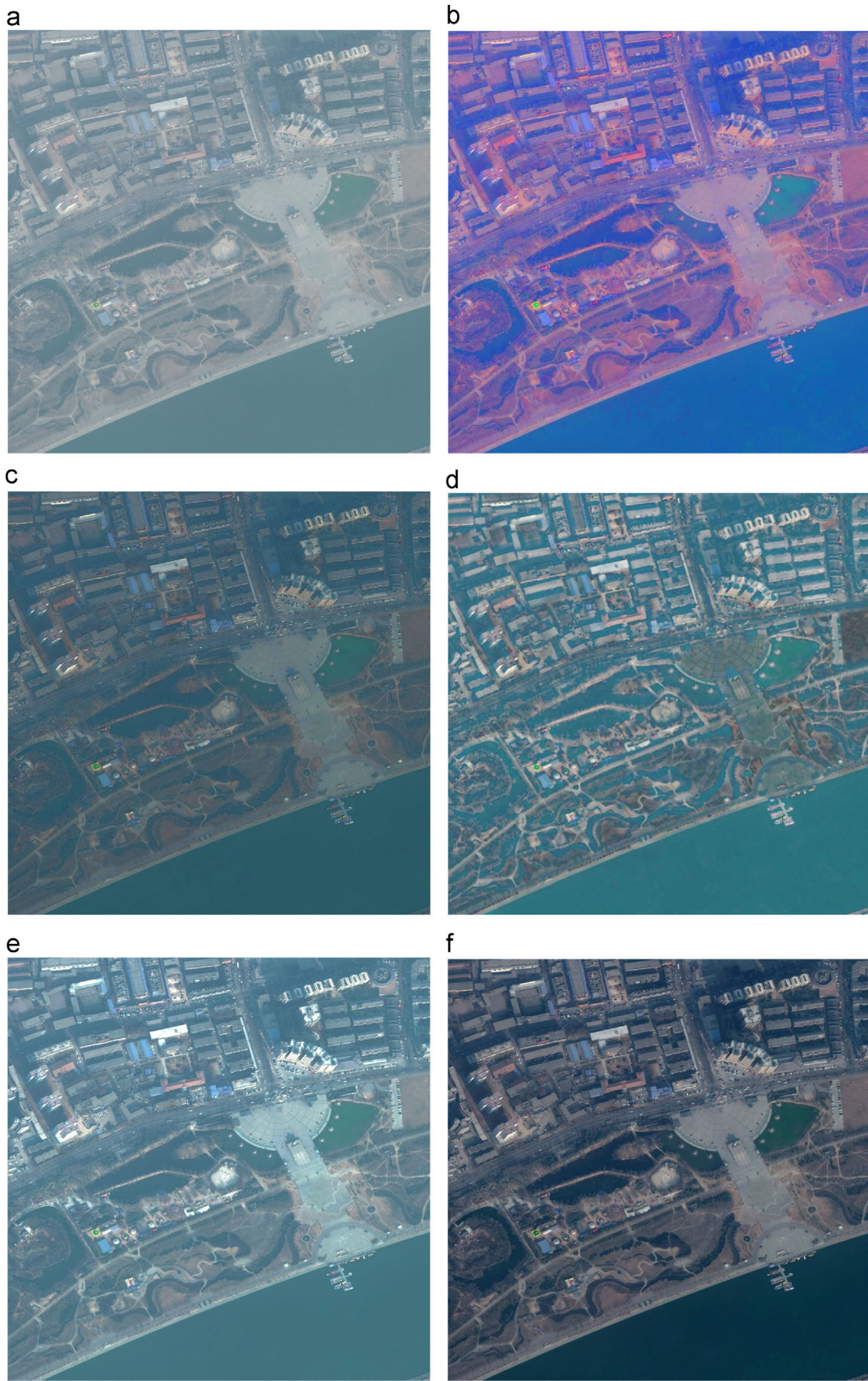
Fig. 10. From top to bottom and left to right, the original hazy satellite image and the results obtained by MSR, He et al.'s [16], Tarel's [25] and Fattal's [14] and our method. (For interpretation of the references to color in this figure, the reader is referred to the web version of this article).
