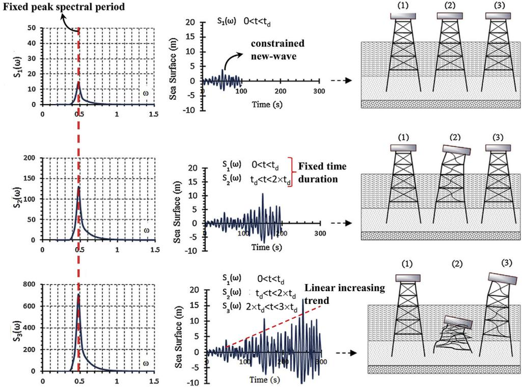
Fig. 1. The hypothetical test showing the concept of EWA method [9].
