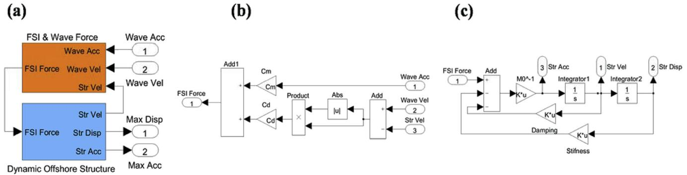
Fig. 9. MATLAB SimuLink blocks (a) SimuLink model (b) “FSI & Wave Force” block (c) “Dynamic Offshore Structure” block.
