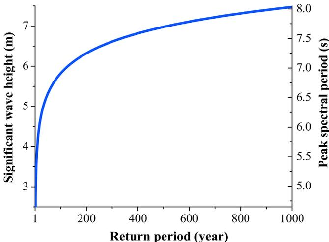
Fig. 6. Significant wave height and its corresponding peak spectral period via return period in the Persian Gulf.
