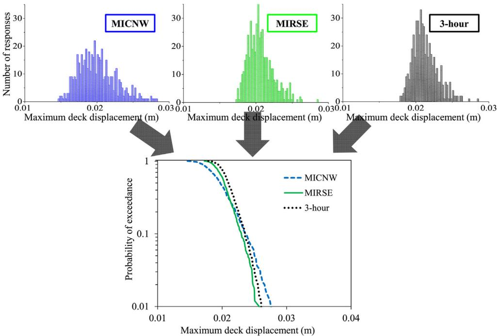
Fig. 10. Extreme deck displacement distribution and its cumulative probability distribution for MICNW, MIRSE and 3-h records (2-year return period).
