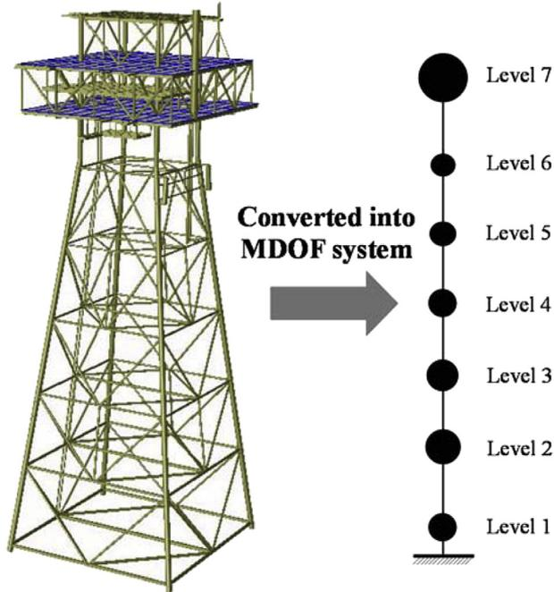
Fig. 8. Resselat platform and its simplified MDOF system.
