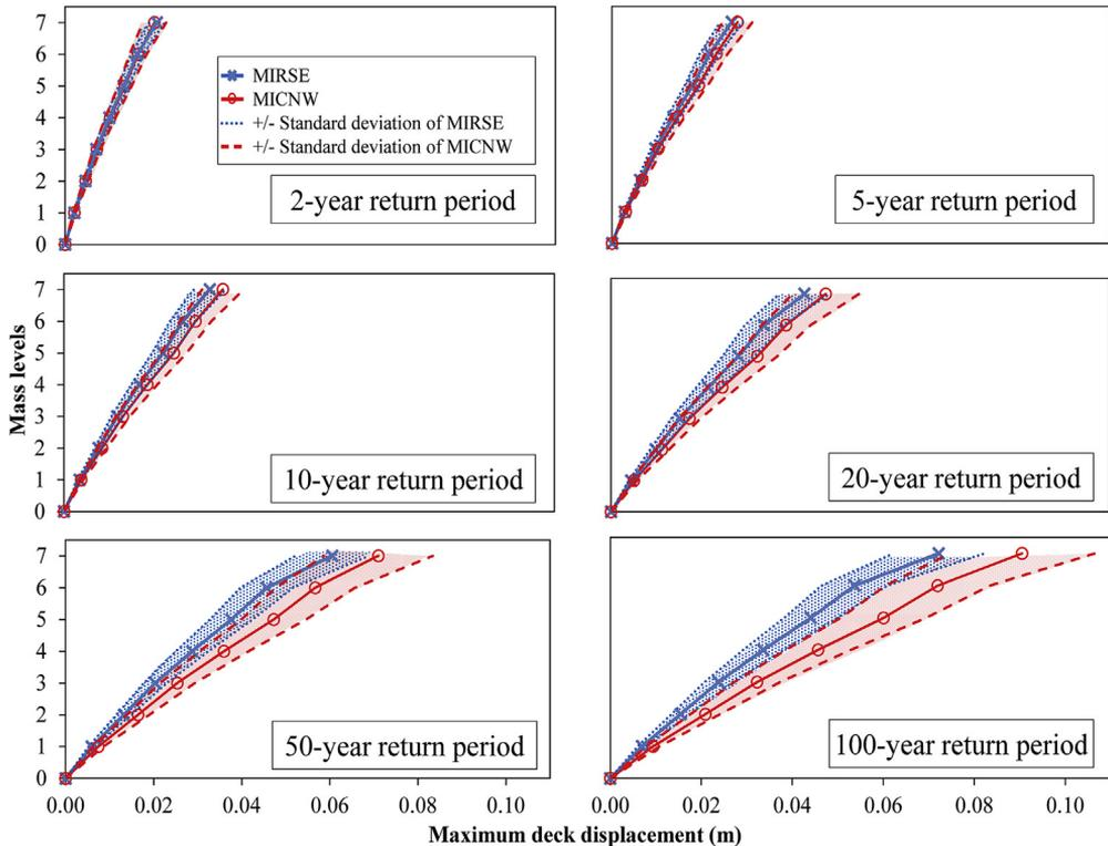
**Fig. 12.** 50% exceedance of maximum displacements in all mass levels for 3-h, MIRSE and MICNW series.
