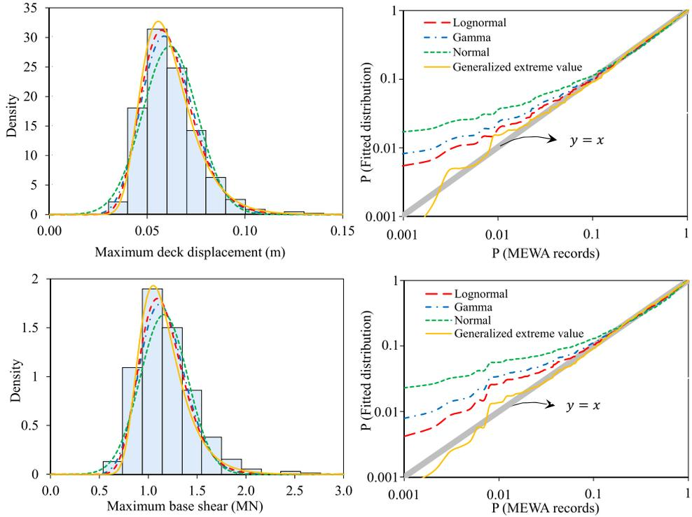
Fig. 14. Different distributions fitted to the sample data from the results of MICNW records.
