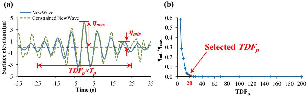
Fig. 5. (a) Defining parameters of  $TDF_p$  criterion for new-wave and constrained new-wave theories and (b) the ratio of minimum and maximum amplitudes for different  $TDF_p$ s.
