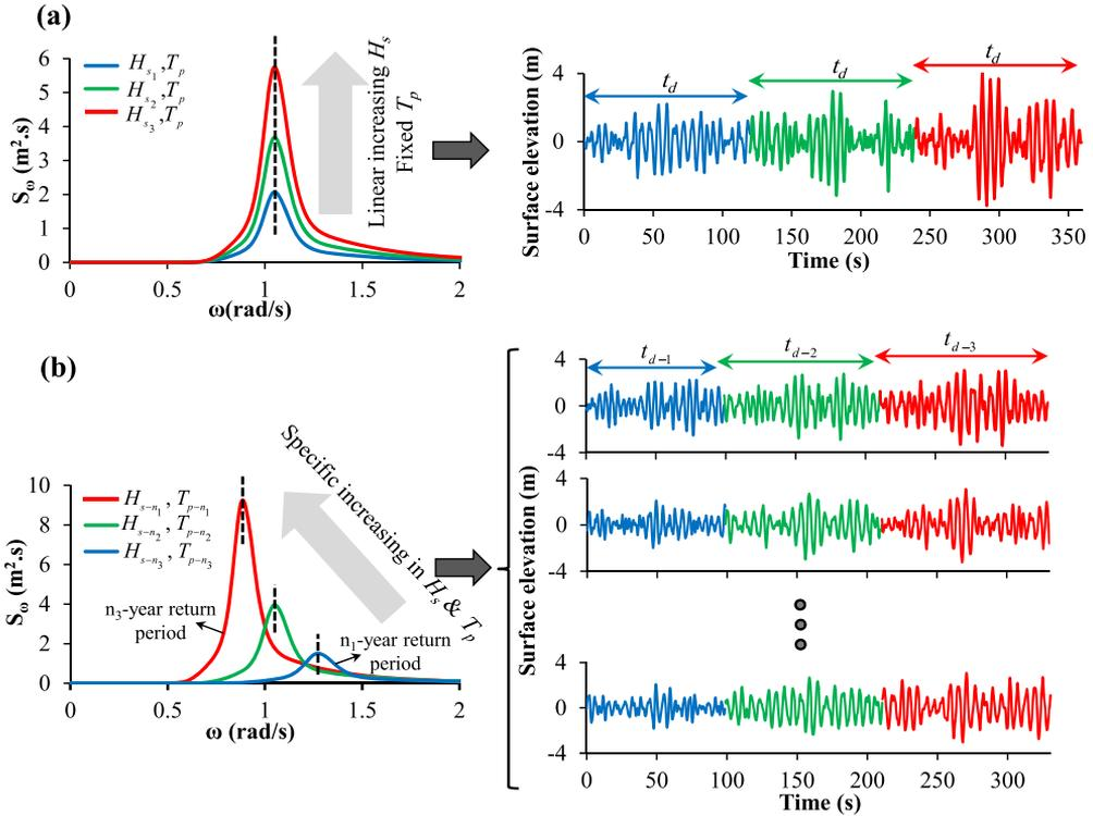
Fig. 2. A sample of (a) EWA and (b) MEWA records and their corresponding spectrums.
