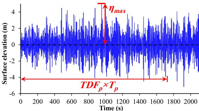
Fig. 3. A record of random wave theory and the maximum amplitude  $\eta_{\max}$ .
