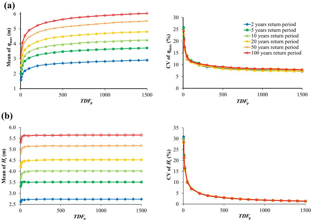
Fig. 4. Mean and CV of (a)  $\eta_{max}$  and (b)  $H_s$  for random wave records and different return periods.
