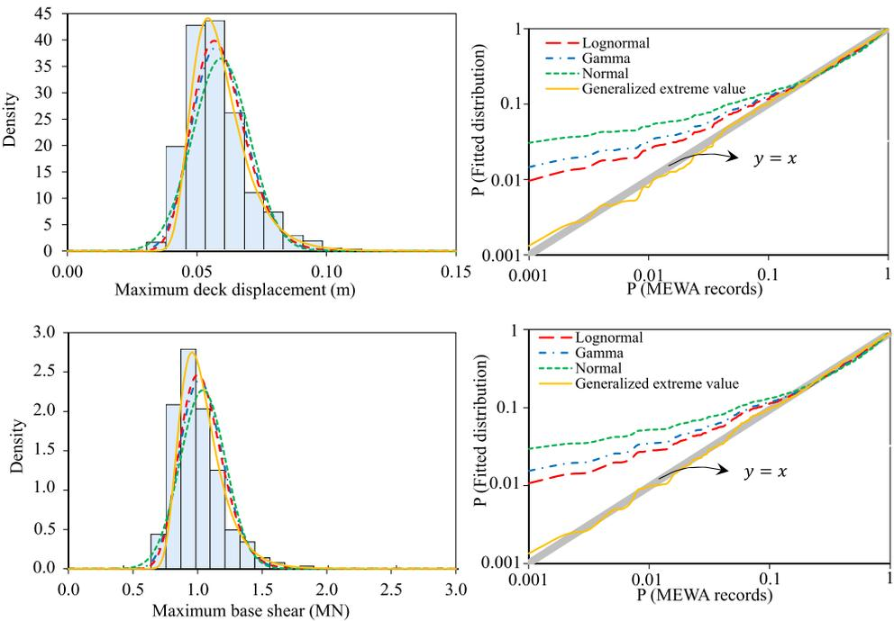
Fig. 13. Different distributions fitted to the sample data from the results of MIRSE records.
