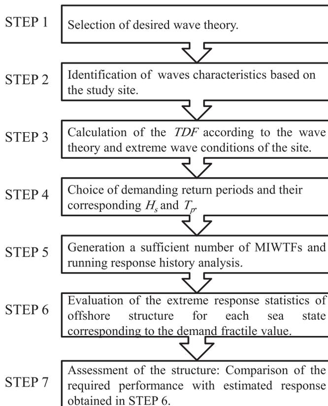
Fig. 16. Recommended procedure of the MEWA method for stochastic estimation of the response of offshore platform.
