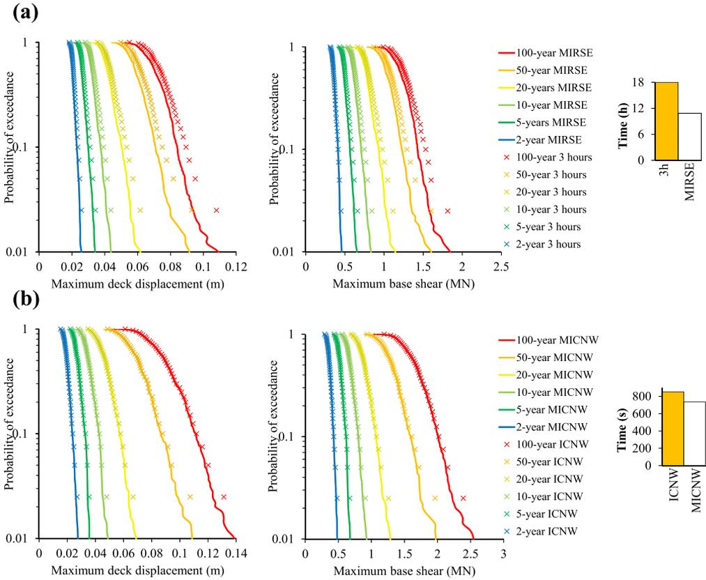
Fig. 11. Comparison of results and total time of analysis (a) MIRSE and 3-h simulation and (b) MICNW and ICNW.
