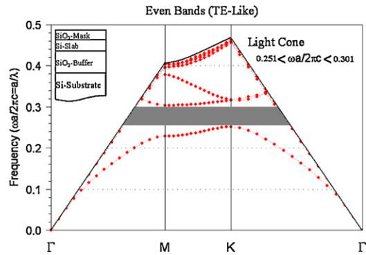
Fig. 1. Dispersion curve for PC with  $R = 115$  nm and  $a = 420$  nm excited by light with TE mode.
