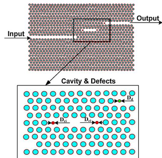
Fig. 2. A structure with a single resonance cavity, one input waveguide and one output waveguide accompanying with shown point defects.
