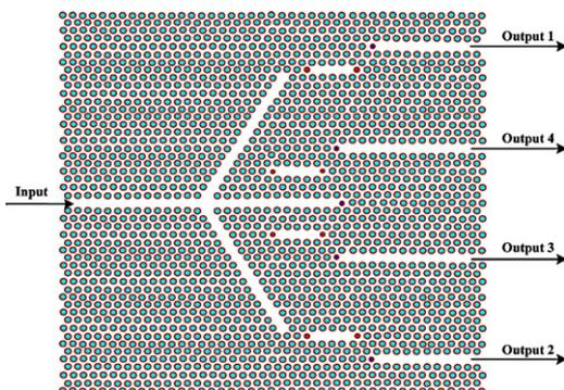
Fig. 4. Four channel demultiplexer based on modified Y-Branch structure.
