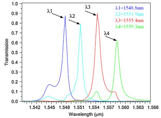
Fig. 5. Representation of the demultiplexer output channels at  $\lambda_1$ ,  $\lambda_2$ ,  $\lambda_3$  and  $\lambda_4$  wavelengths.
