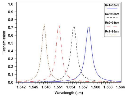
Fig. 3. The ratio of wavelength variations of the output waveguide due to various amounts of  $Dc_i$  in the resonance cavity.
