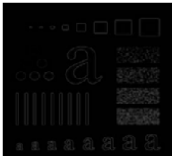
Fig. 19: result of BHPF of order 2 with D_0 = 160
