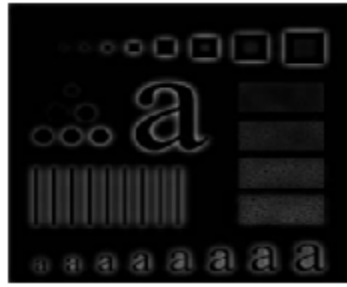
Fig. 17: result of BHPF of order 2 with D_0 = 30
