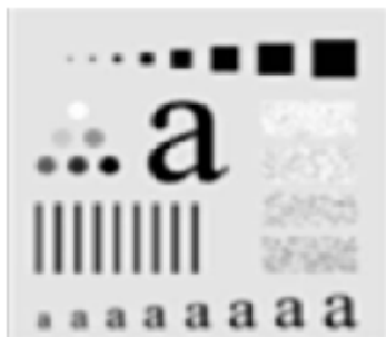
Fig. 13: result of filtering with Cutoff frequency set at radius value 60
