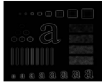
Fig. 18: result of BHPF of order 2 with D_0 = 60
