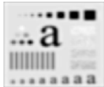
Fig. 12: result of filtering with Cutoff frequency set at radius value 30
