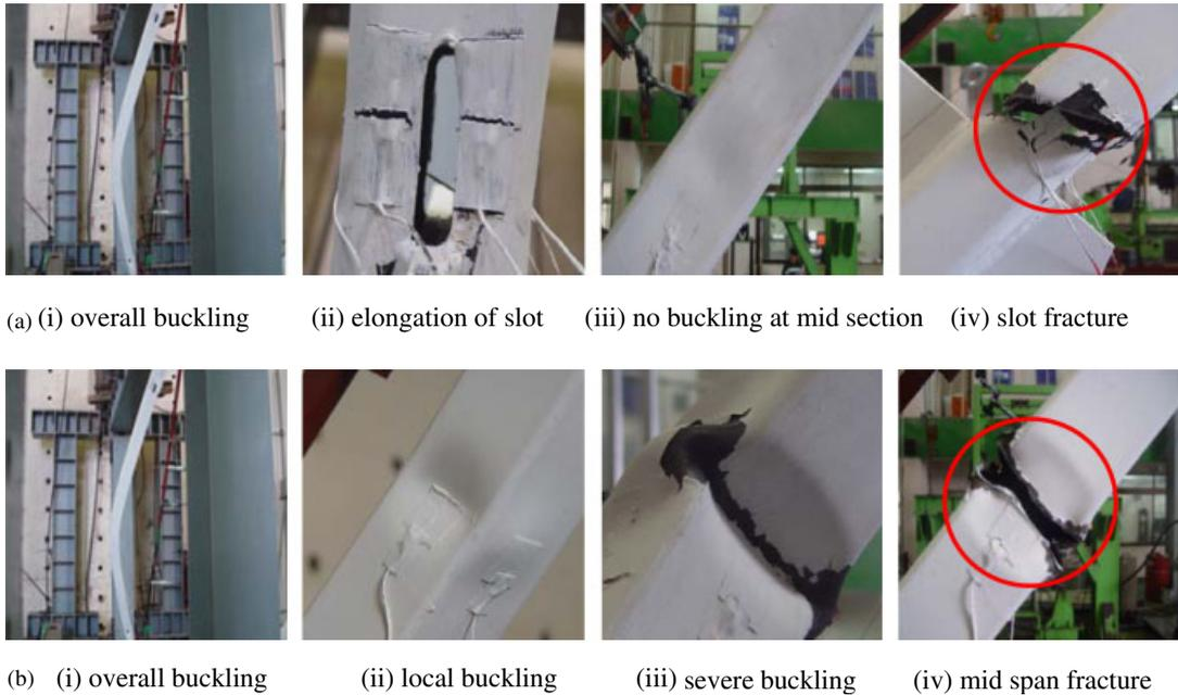
Figure 6. Buckling and fracture of specimens: (a) S 90-8 and S 69-11; and (b) R 90-8 and R 69-11.
