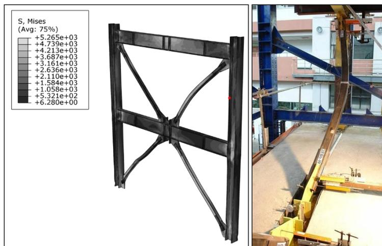
Fig. 6: Deformation between the experimental [22] and FEM simulations.
