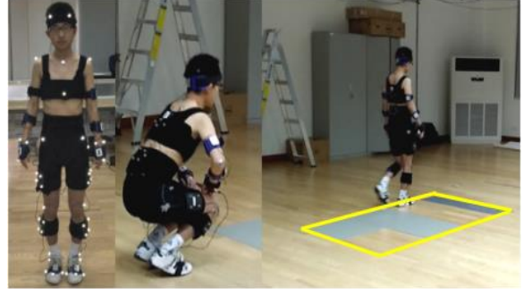
Figure2. (a) Performer puts on the suit with sensors and attaches 65 markers; (b) Squatting and rising experiment; (c) Walking motion experiment
