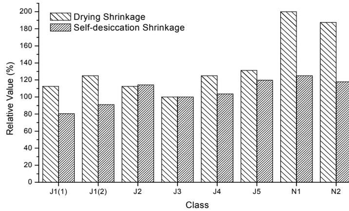
Fig. 5 Comparison between drying shrinkage and self-desiccation shrinkage of concrete with different superplasticizers
