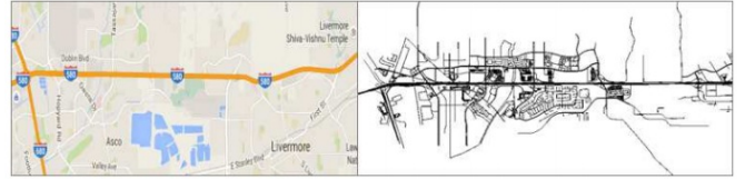
Figure 6. San Jose (California) urban area (left) exported to a VANET network topology by using MOVE/SUMO (right).
