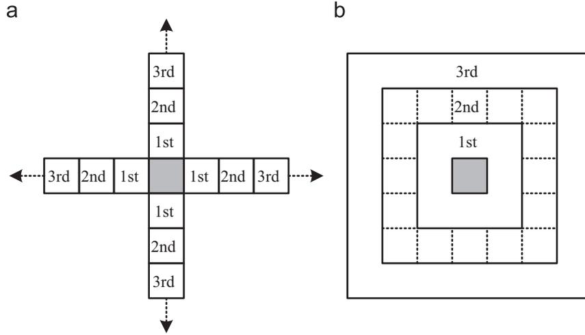
Fig. 2. Employed types of windows; (a) the simplified type for low densities of noise ratio; (b) the full type for high densities of noise ratio.
