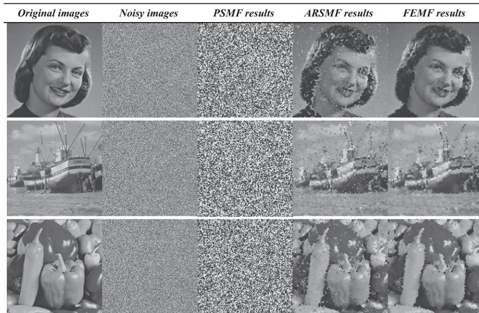
Fig. 6. Noise reduction by each method for different gray-scale images at 98% of noise ratio.
