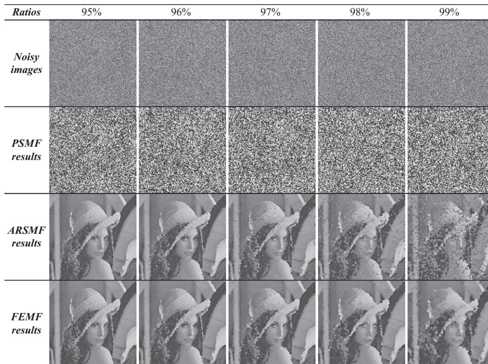
Fig. 5. Noise reduction by each method for Lena images at different noise ratios.
