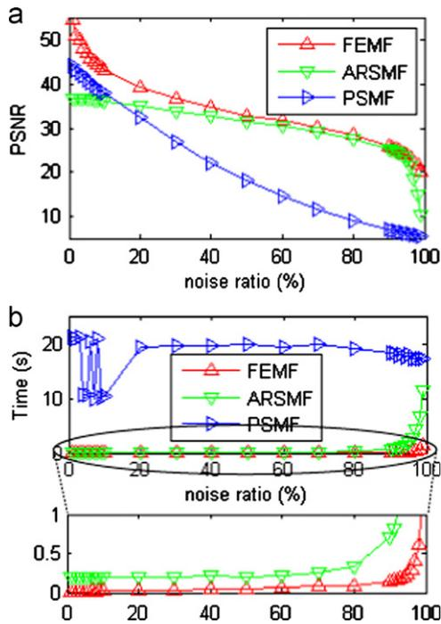
Fig. 4. Comparison of noise reduction methods for (a) quantitative measurement and (b) execution time.
