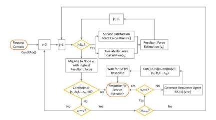
Fig. 1. Migration and service composition process of a requester agent RA(v)
