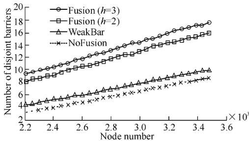
Fig. 9 Number of disjoint barriers vs. number of sensors
