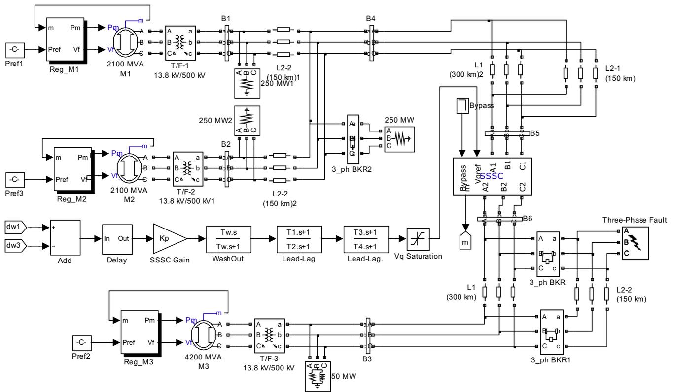
Fig. 13. Developed multi-machine MATLAB/SIMULINK model power system with SSSC.
