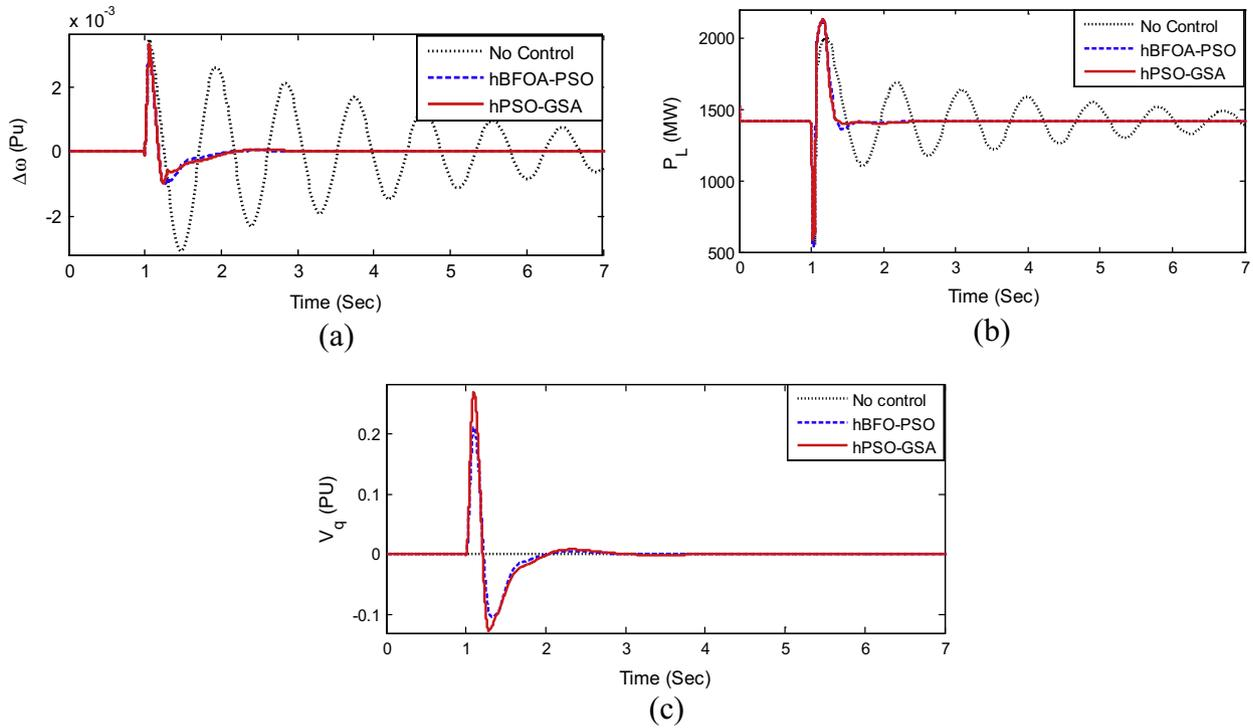
Fig. 8. System response for the case A.1. (a) Speed deviation, (b) tie-line power and (c) SSSC injected voltage.
