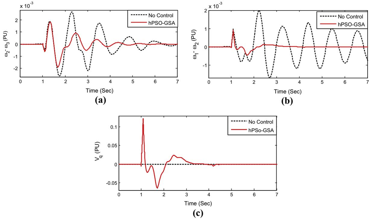
Fig. 14. (a) Inter-area mode of oscillations, (b) local mode of oscillations and (c) SSSC injected voltage, response of the system for B.1 case.
