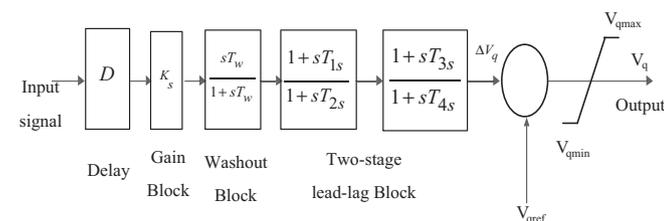
Fig. 2. Structure of SSSC based damping controller.
