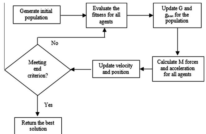
Fig. 6. Flow chart for the proposed hybrid PSO–GSA algorithm.
