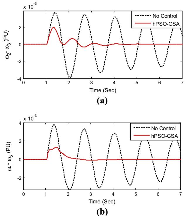
Fig. 16. (a) Inter-area mode of oscillations and (b) local mode of oscillations response of the system for B.2 case.
