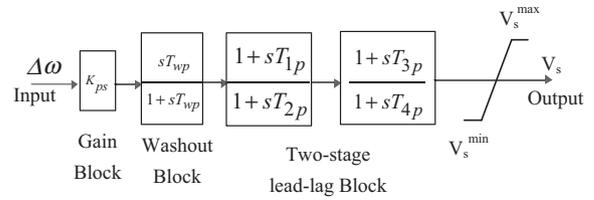
Fig. 3. Structure of power system stabilizer.
