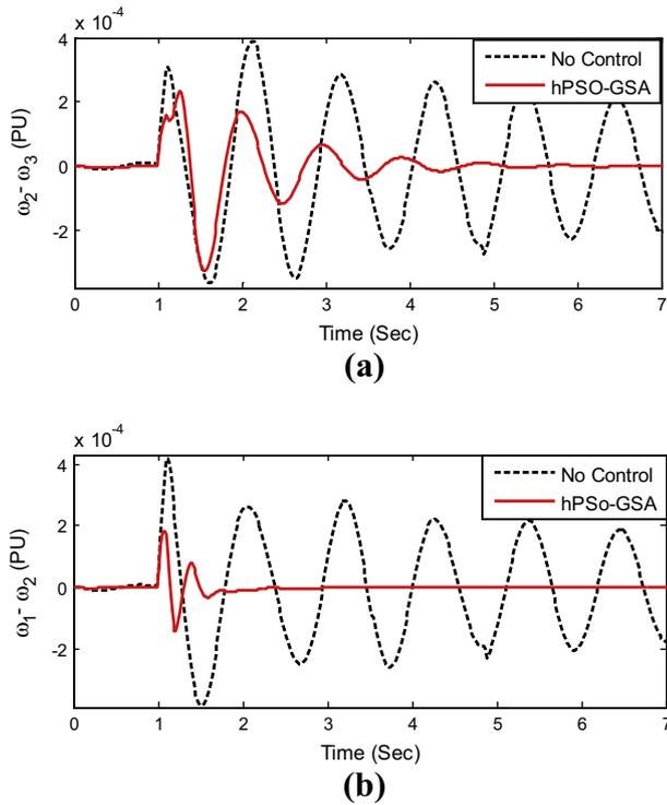
Fig. 17. (a) Inter-area mode of oscillations and (b) local mode of oscillations response of the system for B.3 case.
