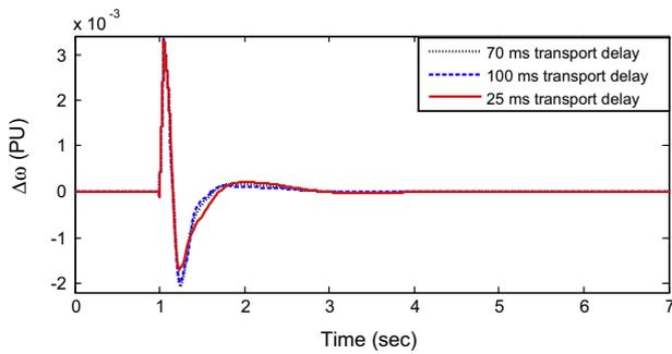
Fig. 9. Speed deviation response of the system with variation of signal transmission delays.
