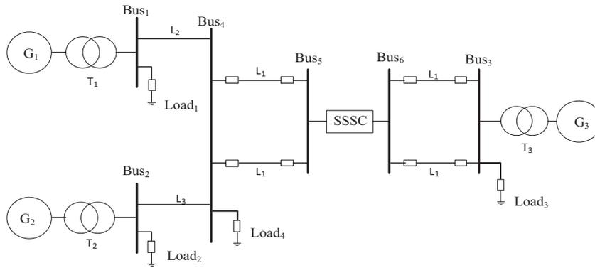
Fig. 12. An example of a multi-machine power system.
