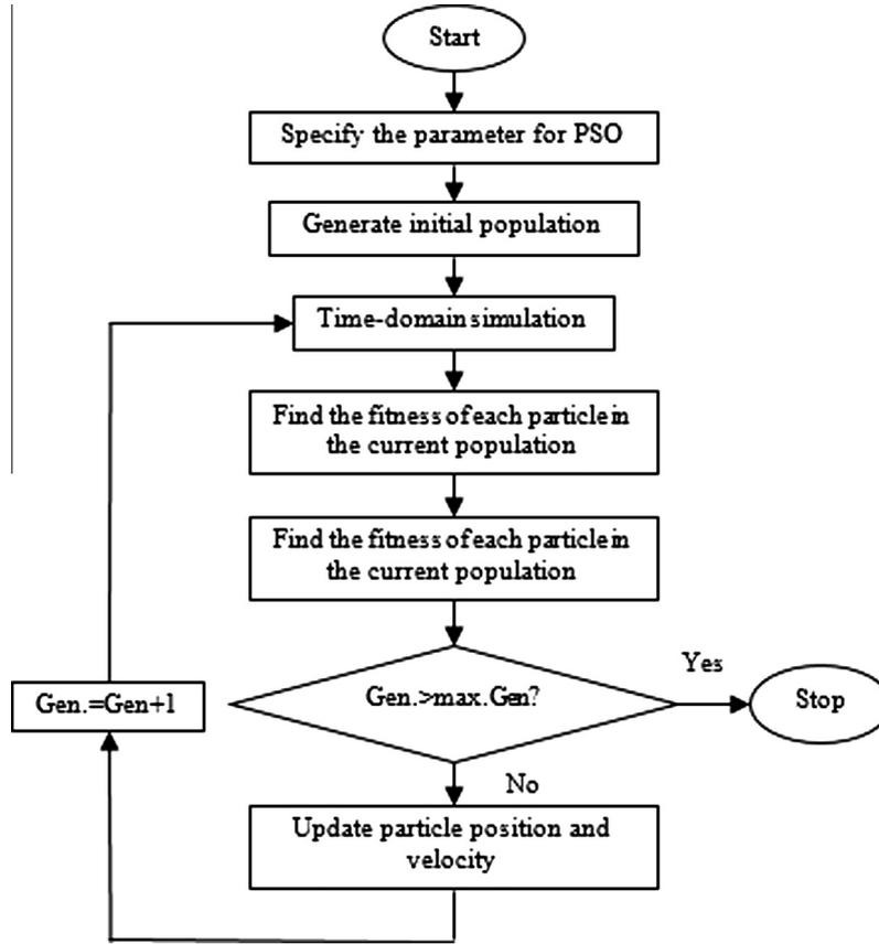
Fig. 4. Flow chart for particle swarm optimization.
