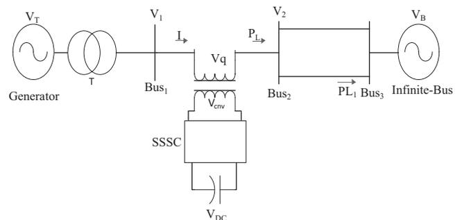
Fig. 1. SMIB system installed with SSSC.
