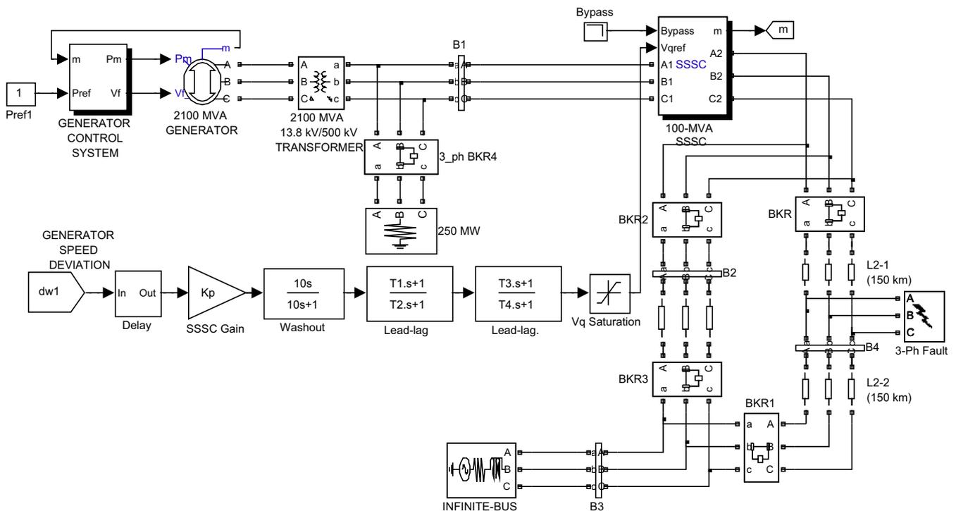
Fig. 7. MATLAB/SIMULINK model of SMIB power system with SSSC.
