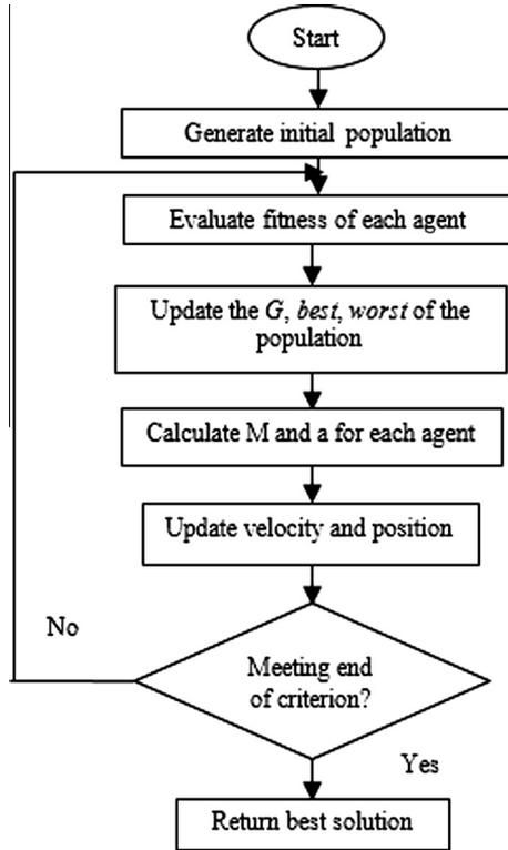
Fig. 5. Flow chart for gravitational search algorithm.
