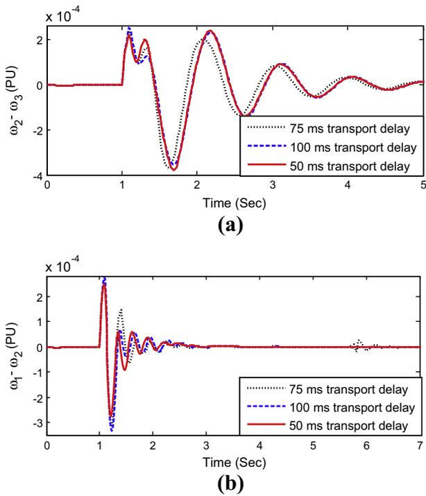
Fig. 15. (a) Inter-area mode of oscillations and (b) local mode of oscillations response of the system in variation with signal transmission delays.
