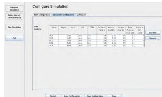
Snapshot-3 This configure simulation define the data center with different region having the operation system linux and also define the cost of every virtual machine.
