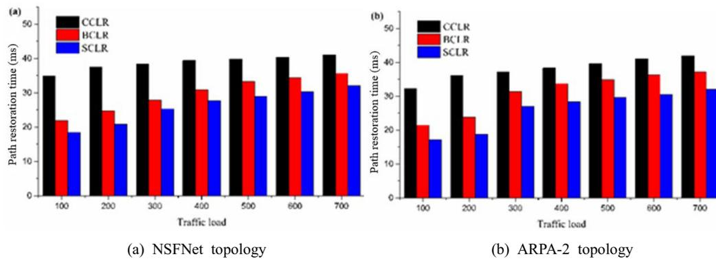
Fig. 8. Path restoration time of CCLR, BCLR, and SCLR schemes in (a) NSFNet. (b) ARPA-2.
