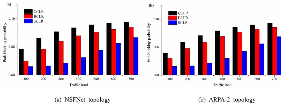
**Fig. 7.** Path blocking probability of CCLR, BCLR, and SCLR schemes in (a) NSFNet. (b) ARPA-2.
