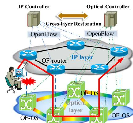
Fig. 1. The architecture of OpenFlow-enabled software defined networking based on IP over optical networks.
