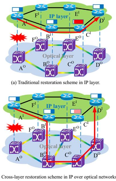
**Fig. 3.** Illustration of different schemes for the service restoration when cross-layer link failure occurs.
