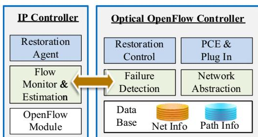
Fig. 2. The functional model of the controllers in software defined networking architecture for cross-layer restoration.
