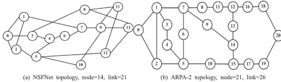
**Fig. 6.** Network topologies NSFNET (a) and ARPA-2 (b). The nodes shown in (a) and (b) are only the IP routers that are interconnected to optical transport network elements. Other intermediate IP routers are omitted in the network diagrams and calculations.
