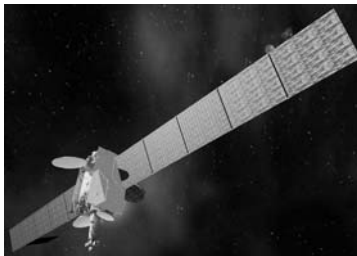
SS/Loral 1300S 19 kW 6200 kg at launch
